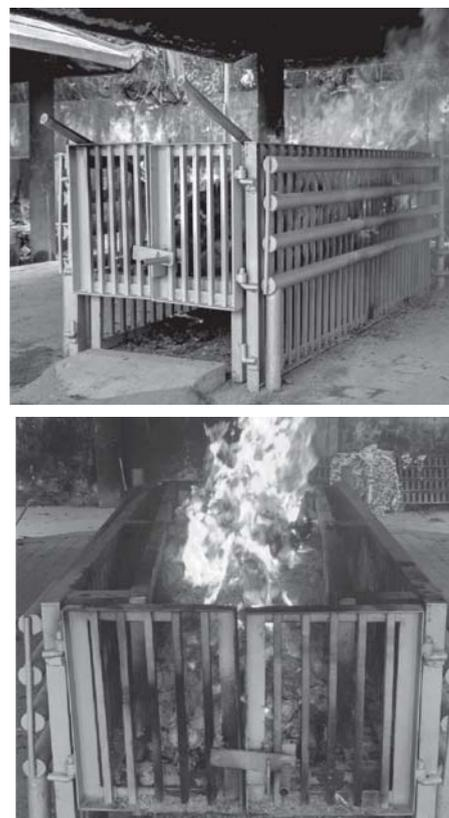
**Fig. 3:** ICAR CIRCOT rectangular shape (top) and trapezoidal shape (bottom) crematoriums in operation at Ambazari Ghat, NMC, Nagpur
