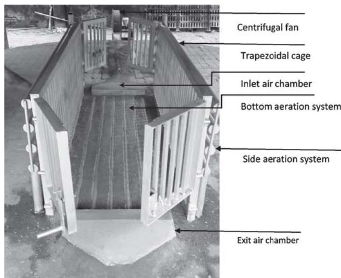
**Fig.1.** ICAR-CIRCOT briquette-based crematorium
