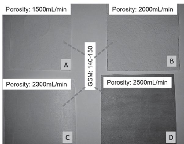
**Fig. 3 :** Sheath materials of different porosity used for the experiment
