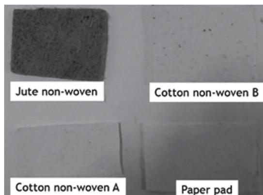
**Fig. 2 :** Core materials used for the experiment
